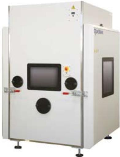
The Typhoon 2.5 is Qualmark's most popular chamber. With a 30" x 30" vibration table, it is just the right size for the vast majority of Highly Accelerated Life Testing (HALT) applications, and many Highly Accelerated Stress Screening (HASS) applications. The table can be mounted in an upper or lower position, to suite your product and ergonomic needs.
